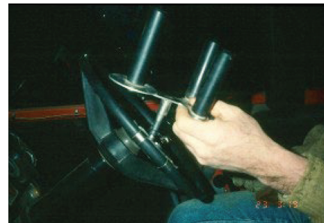
A Modified Steering Wheel is an option for farmers who have difficulties controlling traditional steering wheels on farm equipment.
