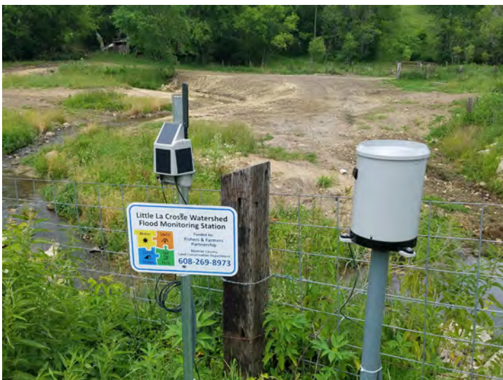
Monroe County has installed monitoring stations at stream crossings with flood histories. Data generated is fed to the National Weather Service to support flood alerts, and also generates stream data for researchers.
