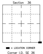
All distances are shown in U.S. Survey Feet. Bearings are for tie reference purposes only. Coordinates were derived from RTK GNSS procedures. Corner I.D. <u>SE 36</u>
