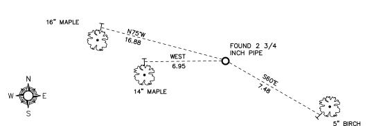
All distances are shown in U.S. Survey Feet. Ties are to 60D nails set in trees. Bearings are for tie reference purposes only. Coordinates were derived from RTK GNSS procedures.
