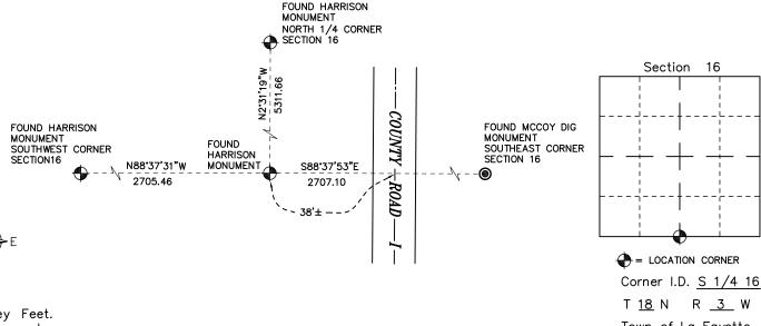
All distances are shown in U.S. Survey Feet. Bearings are for tie reference purposes only. Coordinates were derived from RTK GNSS procedures. Town of La Fayette Monroe County, WI.
