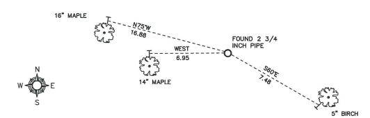
All distances are shown in U.S. Survey Feet. Ties are to 60D nails set in trees. Bearings are for tie reference purposes only. Coordinates were derived from RTK GNSS procedures.
