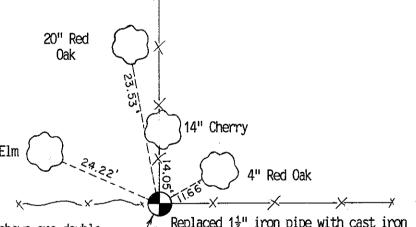
Replaced 1½" iron pipe with cast iron -Harrison marker. Set sign and post on North side of Harrison.
